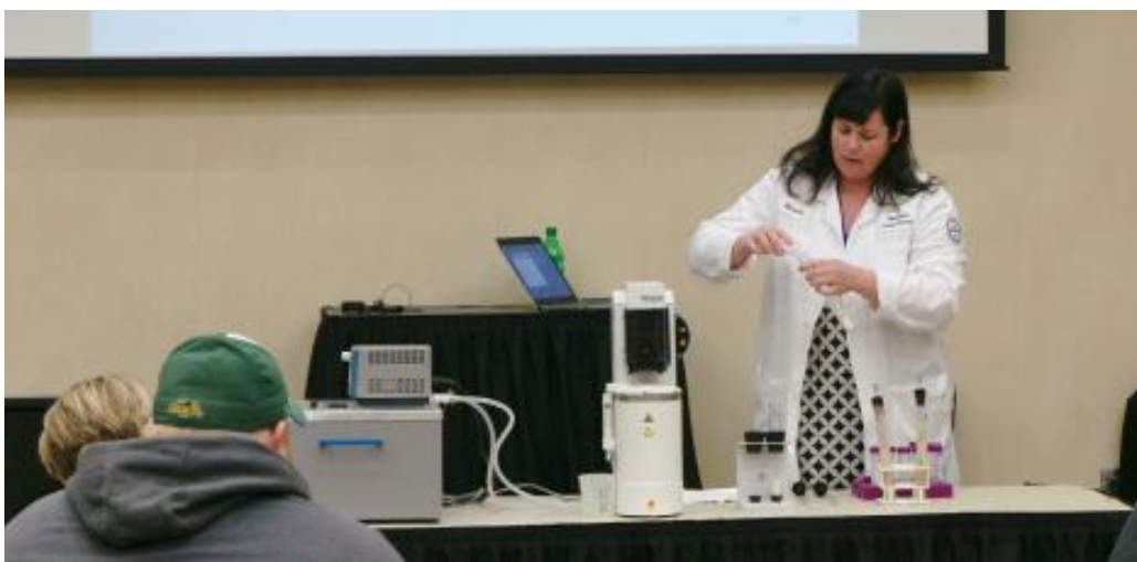
Rhonda Lyne, Physical Scientist at the USDA AMS/ FGIS, demonstrates on the viscometer stirrer rod to see if Alpha-amylase is present.
