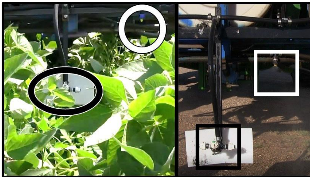
Figure 1. Configuration of the tractor-mounted hydraulic-powered plot sprayer used to apply fungicides in this experiment. Note that two different within-the-canopy booms were built to allow application down the center of both 22 (Crookston study site) and 30 inch (Staples study site)-spaced soybean rows. The within-the-canopy nozzle body (black circle/square) rode approximately 12" from the soil surface and the over-the-top nozzles (white circle/square) rode approximately 8" above the soybean canopy.
